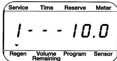
3. Pushing the Extra Cycle Button during a regeneration step will immediately advance the valve to the next regeneration step position.
